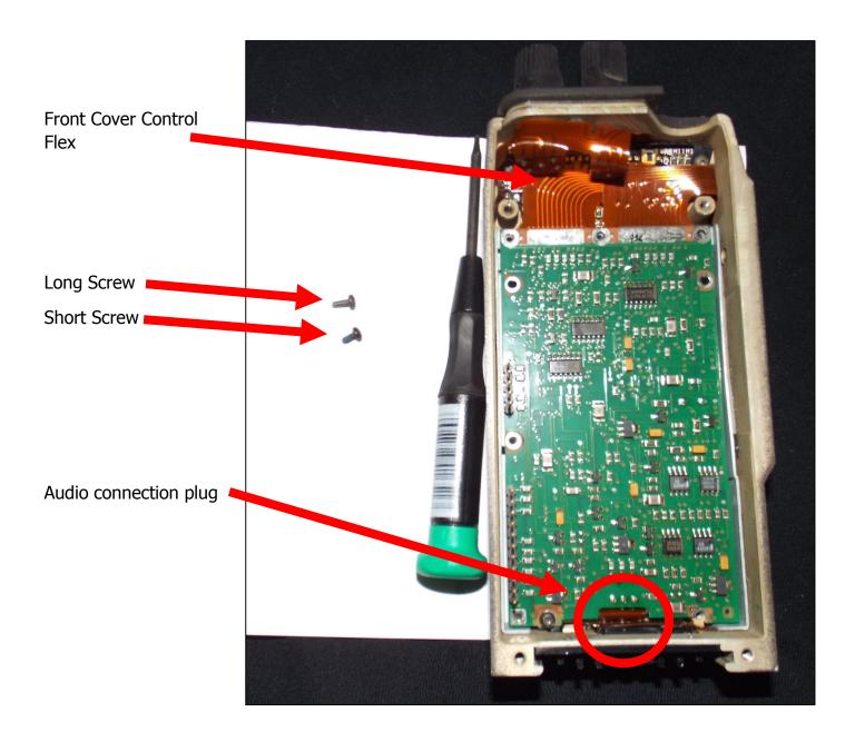
With the screws removed, you can now pivot up the control/logic board and disconnect the audio plug at the bottom of the board.
